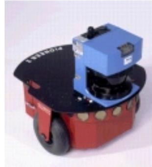
Figure 1: The Pioneer 2 DX mobile robot equipped with an LMS 200 laser scanner.
