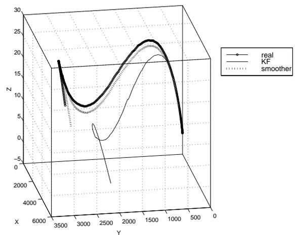
Figure 6: This is an example trajectory in 3D. The thick line (circles) represents the real motion of the vehicle. The thin line is the computed based on the attitude information from the Kalman filter, and the thick dashed is the computed using the attitude information provided by the smoother.
