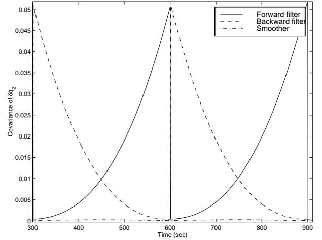
Figure 4: The covariance related to  $q_2$  from the forward filter, backward filter and smoother is shown. At all times the total covariance is lower than either of the corresponding ones calculated from the two filters. Its value remains bounded and varies slightly during the smoothing interval.
