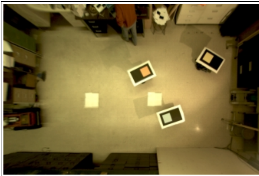
Figure 2. Rectified image of the Pioneer robots with color patches for tracking and identification as viewed from the overhead camera.
