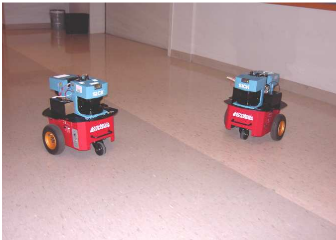
Fig. 4. The robots used in the experiments. Two laser range-finders are installed on each of the robots, to provide a 360° field of view.
