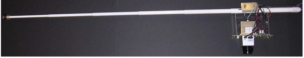
Fig. 4. A view of white cane and hardware. The sensor bay is mounted on the handle portion of the cane. Note that the tip of the cane is unobstructed, and the user maintains the ability to physically sense the world. The weight of the sensor package is approximately 550g.
