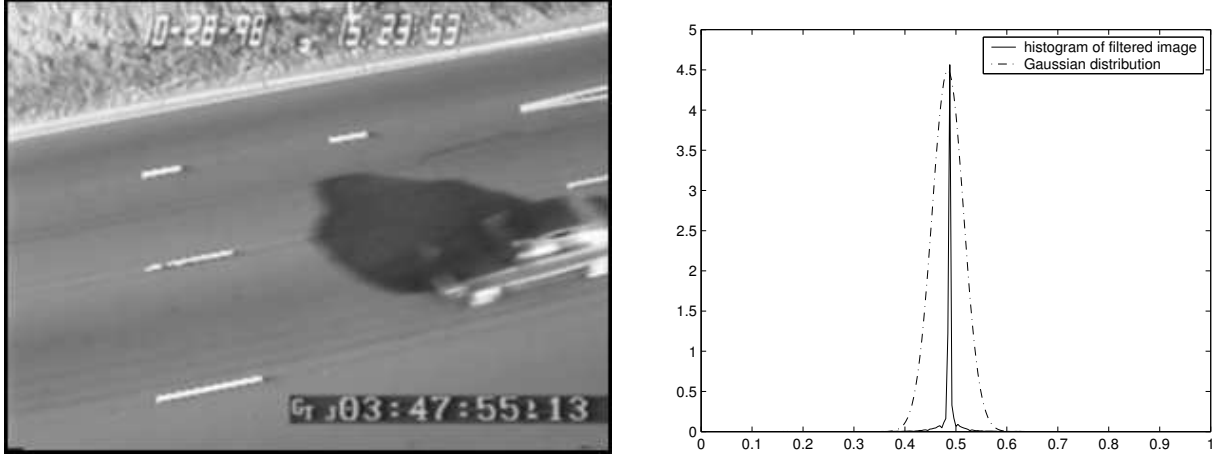
Fig. 1. A frame from our traffic sequence and the resulting histogram of the filter output. The Gaussian has unit variance and has been scaled and shifted to coincide with the peak of the histogram.
