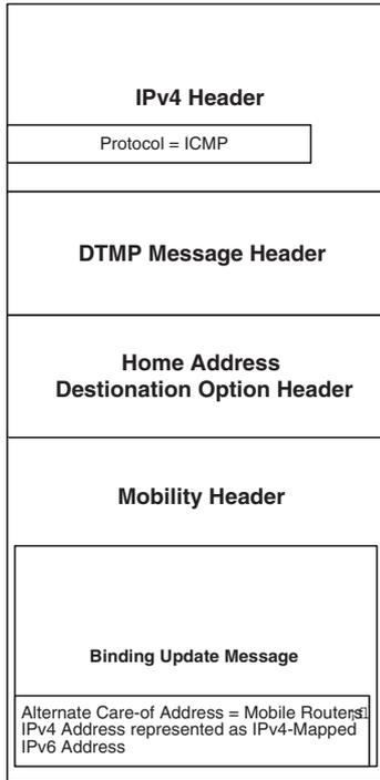
Fig. 5. IPv4 Datagram Layout for IPv6-in-IPv4 Tunnel Management
