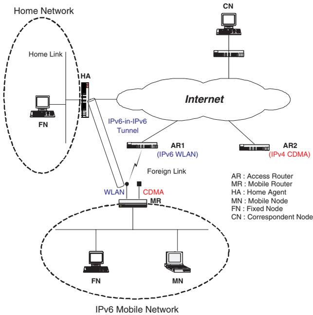
Fig. 1. IPv6 Mobile Network connected to IPv6 Access Network
