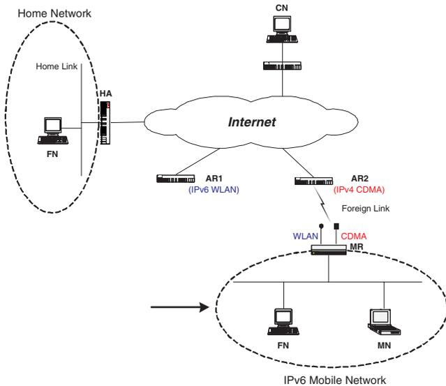
Fig. 2. IPv6 Mobile Network moving into IPv4 Access Network
