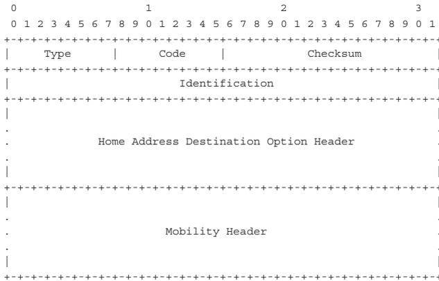
Fig. 6. Dynamic Tunnel Management Protocol (DTMP) Message Format
