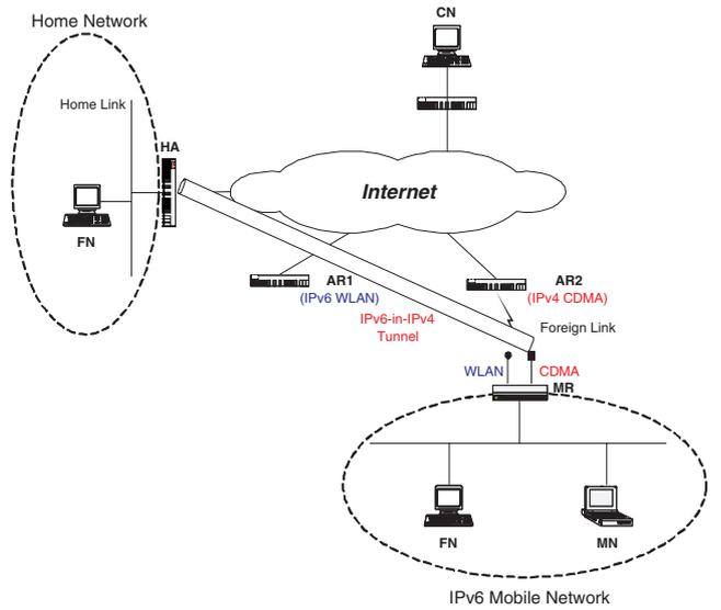
Fig. 3. Setup of IPv6-in-IPv4 Tunnel
