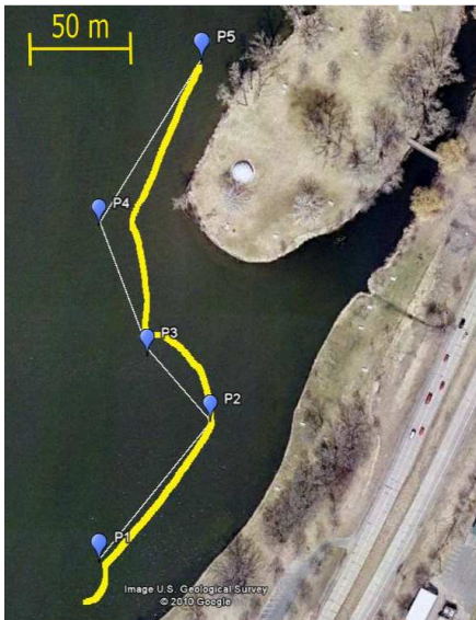
(a) The GPS trail is made in yellow along with the reference trajectory in white. The total distance covered from the first to the last waypoint was about 304m in 16 mins.
