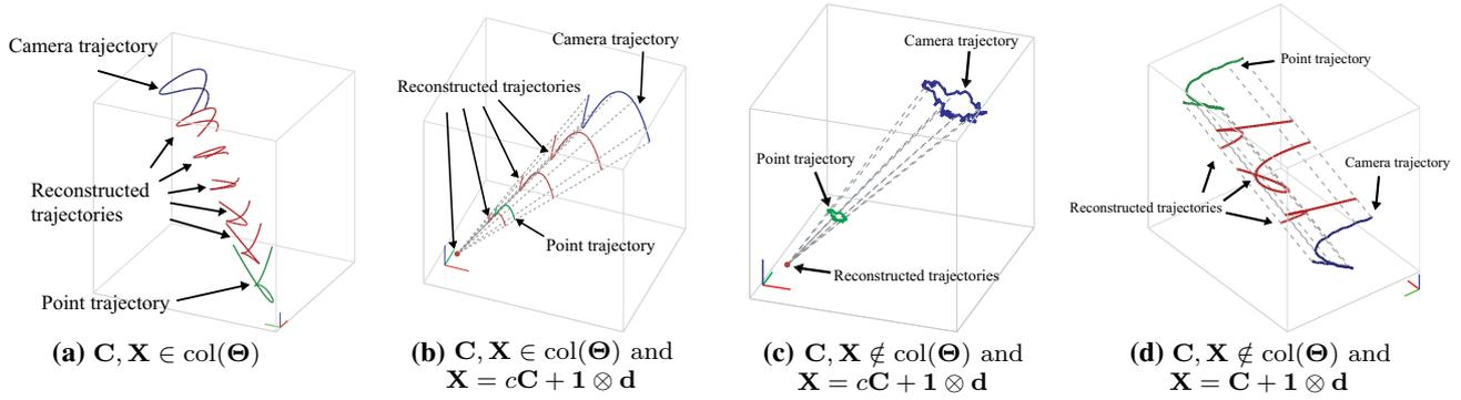
**Fig. 5** We illustrate unsolvable systems that produce an infinite number of solutions or a trivial solution. **a** Trajectory reconstruction is ambiguous when  $\mathbf{C}, \mathbf{X} \in \text{col}(\Theta)$  because there exists  $\text{null}(\mathbf{Q}\Theta)$ , which is an unsolvable system. Plausible reconstructed trajectories that satisfy Eq. (7) are illustrated. **b** Plausible reconstructed trajectories that satisfy
