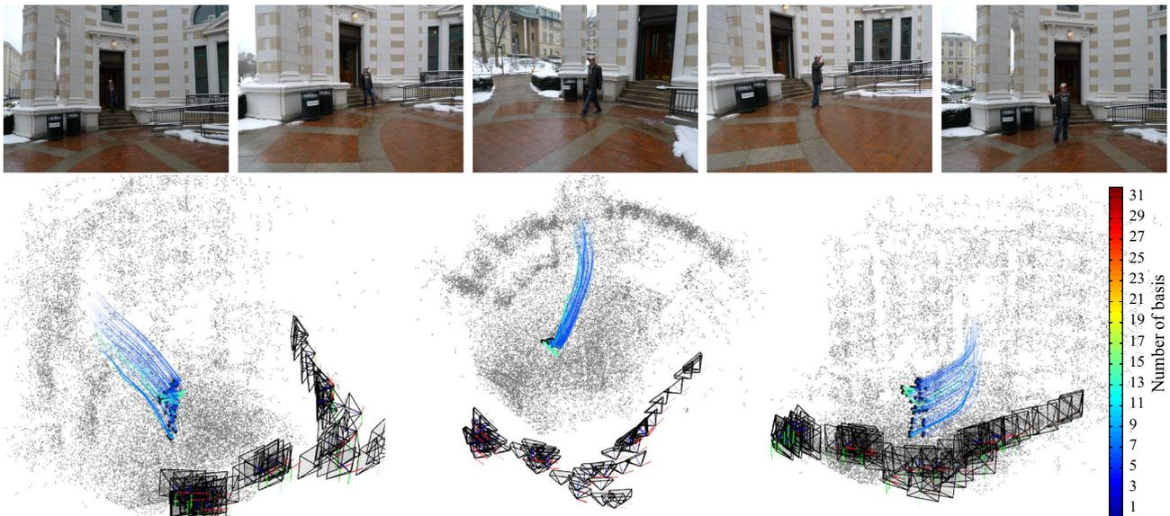
**Fig. 18** Results of the greeting scene. *Top row* sampled image input and *bottom row* reconstructed trajectories in different views. The number of basis vectors is color-coded
