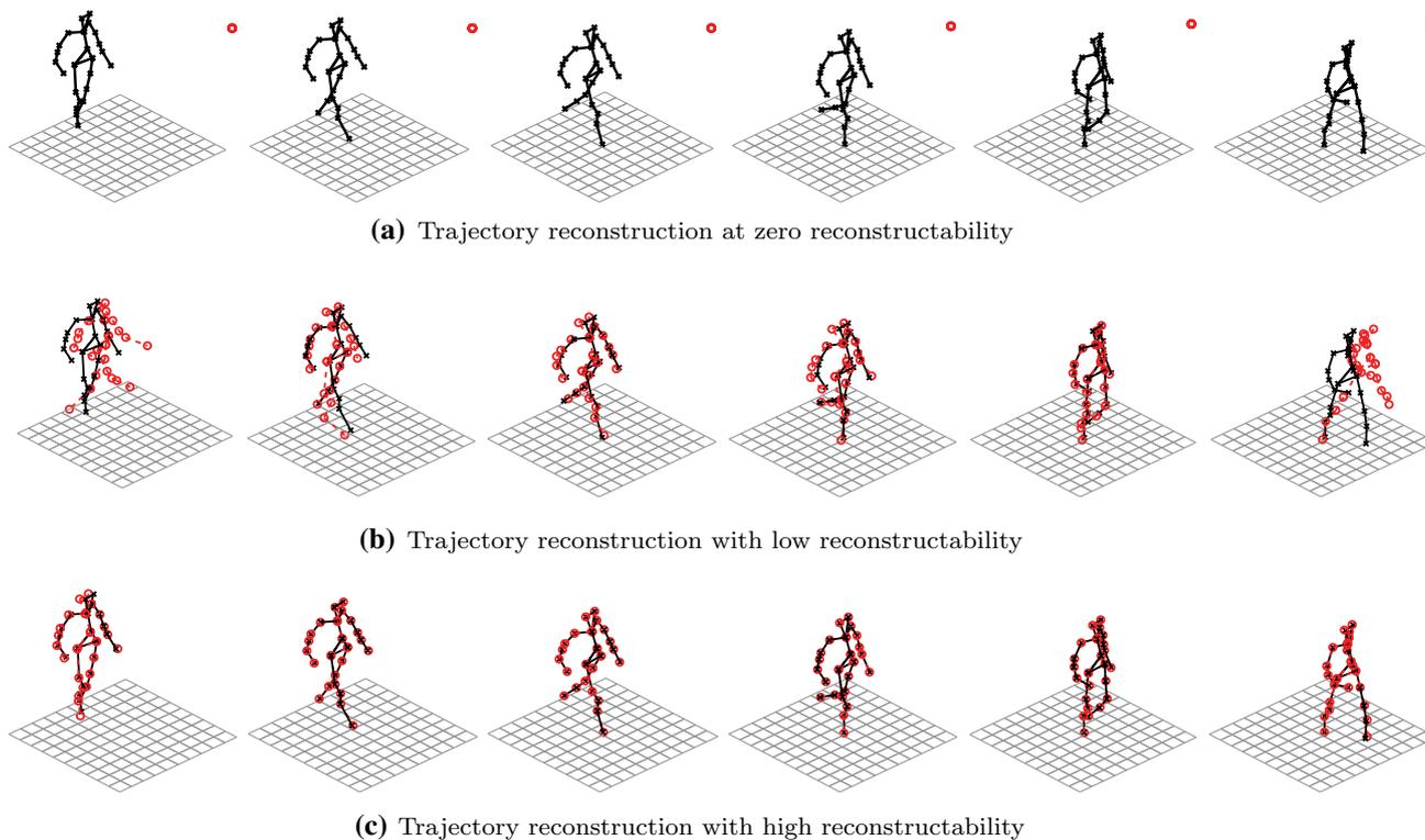
**Fig. 9** Qualitative comparison of trajectory reconstruction from various reconstructability. *Black* ground truth, *red* reconstructed trajectory. **a** Zero reconstructability,  $\eta = 0$ . The relative camera trajectory is stationary and the reconstructed trajectory is exactly the same as the
