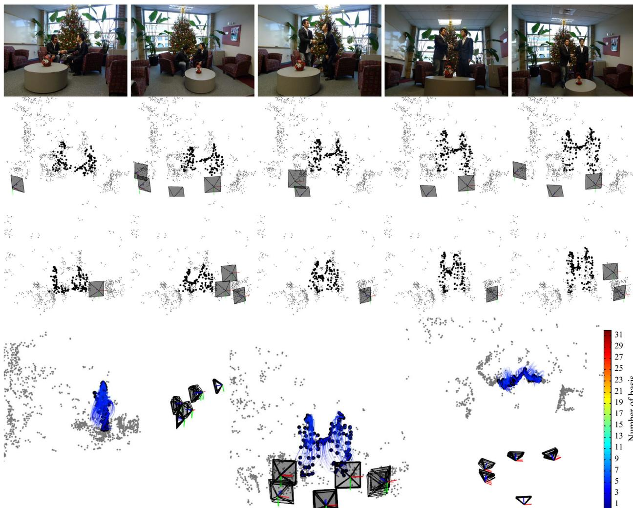
**Fig. 16** Results of the handshake scene. *Top row* sampled image input, *second* and *third row* five snap shots of 3D reconstruction in different views, and *bottom row* reconstructed trajectories. The number of basis vectors is color-coded
