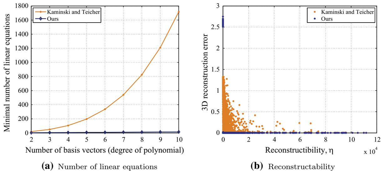
**Fig. 11** **a** The minimal number of linear equations increases exponentially as the degree of polynomial (degree of motion) increases for the method by Kaminski and Teicher (2004) while it increases linearly for our method. This computationally precludes them to reconstruct a tra-
