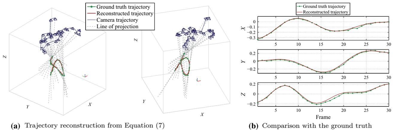
**Fig. 2** We reconstruct a trajectory using linear least squares. **a** The reconstructed trajectory is illustrated in two views. The trajectory, which is represented by a linear combination of trajectory basis vectors, passes through all lines of projections. The *blue pyramids* are camera poses. **b**
