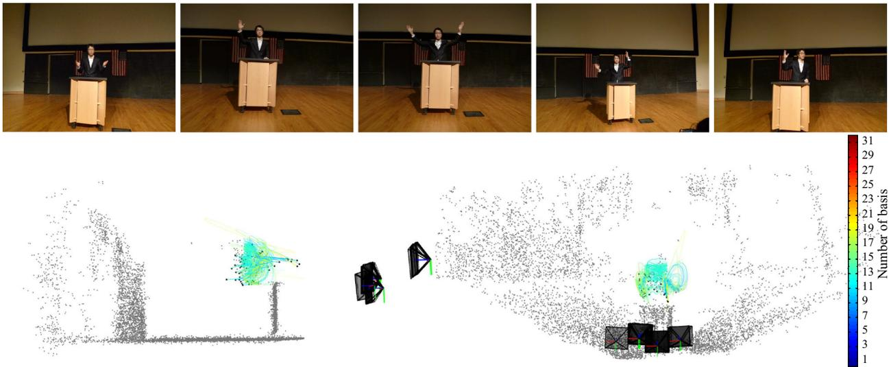
**Fig. 17** Results of the speech scene. *Top row* sampled image input, and *bottom row* reconstructed trajectories in different views. The number of basis vectors is color-coded
