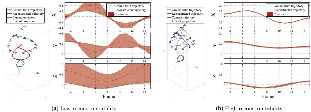
**Fig. 7** The stability of trajectory reconstruction depends on reconstructability. We reconstruct the same point trajectory with the same camera location but with different ordering. Note that the DCT trajectory basis vectors are used for reconstruction. **a** The order of capture forms a smooth camera trajectory (left column), which results in low reconstructability ( $\eta = 0.77$ ) as the camera trajectory can be well represented by the DCT trajectory basis vectors. The reconstructed point
