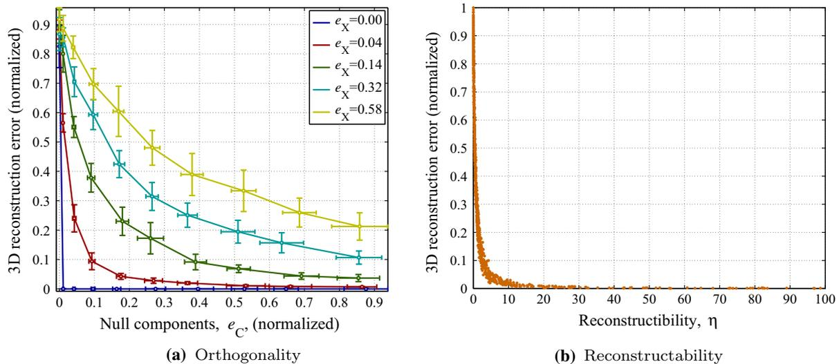
**Fig. 6** **a** As the null component of the camera trajectory  $e_C$  decreases, the solution of Eq. (7) deviates from the ground truth. **b** The reconstructability  $\eta$  provides the degree of interference between the camera
