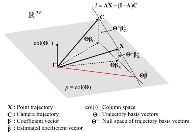
**Fig. 4** Geometric illustration of the least squares solution of Eq. (7). The trajectory  $\Theta \widehat{\boldsymbol{\beta}}$  is placed at the intersection between the hyperplane  $l$  containing the camera trajectory space and the point trajectory, and the  $p$  space spanned by the trajectory basis vectors,  $\text{col}(\Theta)$
