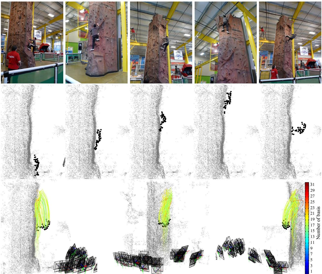
**Fig. 15** Results of the rock climbing scene. *Top row* sampled image input, *second row* five snap shots of 3D reconstruction of motion of the rock climber, and *bottom row* reconstructed trajectories in different views. The number of basis vectors is color-coded
