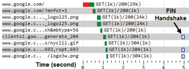
Figure 1: Waterfall diagram of loading `www.google.com` on LTE. ■=TCP Handshake ■=Object Transfer □=FIN handshake.
