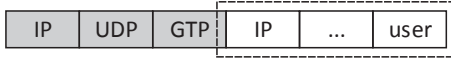
Figure 3: A common configuration of GTP. The user packet is surrounded by dashed line.
