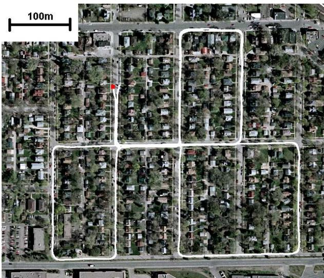
Figure 3. The estimated trajectory overlaid on a satellite image of the area where the experiment took place. The initial position of the vehicle is denoted by a red square.
