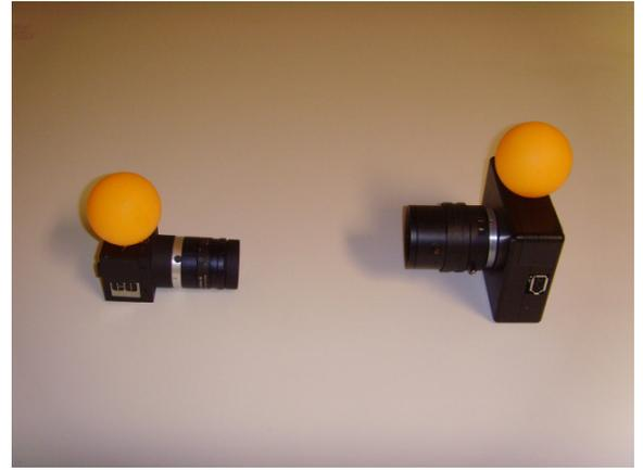
Fig. 7. The two cameras used in the experiment. The Point Grey Dragonfly camera is shown on the right, and the IDS uEye camera is on the left. The two ping-pong balls mounted on top of the two cameras are used as visual targets for measuring the distance and bearing between the two cameras.
