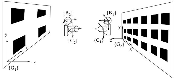
Fig. 8. The experimental setup. The Dragonfly camera,  $\{C_1\}$ , and the uEye camera,  $\{C_2\}$ , are looking at each other. The Dragonfly (uEye) camera uses the known features in  $\{G_1\}$  ( $\{G_2\}$ ) to compute its ego-motion. The Dragonfly (uEye) measures the distance and bearing to the uEye (Dragonfly) by detecting the ping-pong ball  $\{B_2\}$  ( $\{B_1\}$ ).
