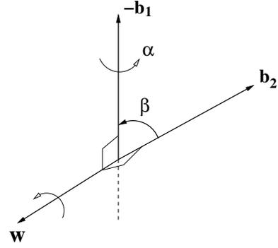
Fig. 4. A rotation that satisfies the constraint  $\mathbf{b}_1 + \mathbf{C}\mathbf{b}_2 = \mathbf{0}$ , where  $\mathbf{w} = \frac{\mathbf{b}_1 \times \mathbf{b}_2}{\|\mathbf{b}_1 \times \mathbf{b}_2\|}$ .
