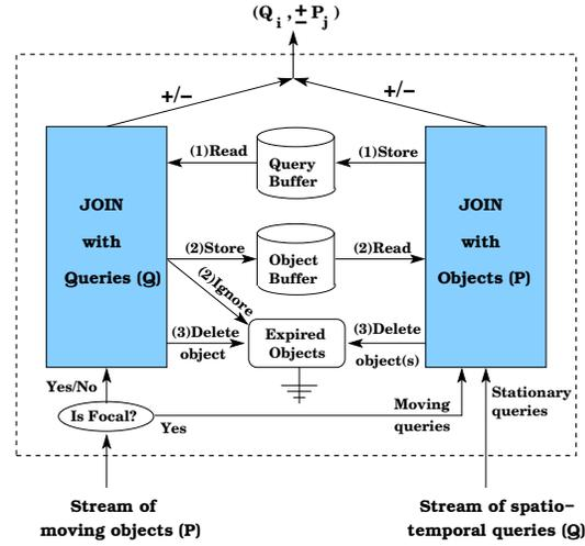
Fig. 6 Shared join operator in SOLE.
