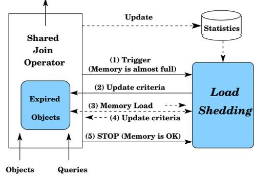
Fig. 9 Architecture of load shedding in SOLE.
