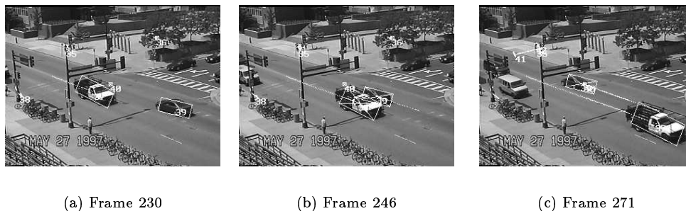
Figure 13: Tracking sequence showing occlusion handling.
