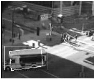
(a) Oriented Bounding Box vs axis aligned box
