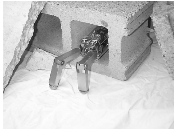
Fig. 1. TerminatorBot climbing through a cinderblock on a mock search-and-rescue mission. Using the narrow-passage gait, TerminatorBot can crawl through spaces that are equal to the width of its body.
