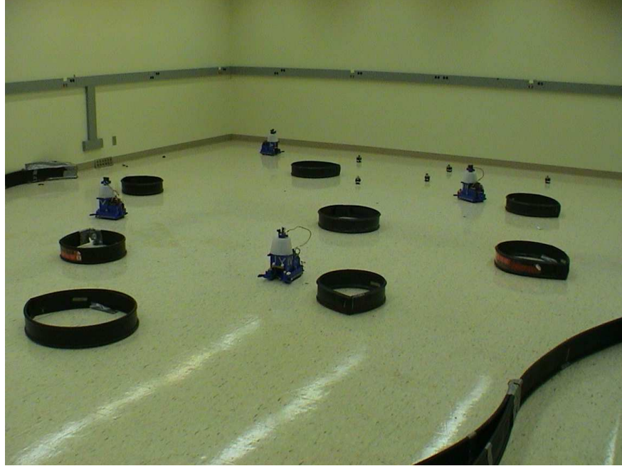
Figure 7: The environment in the communication experiments was approximately 7 m x 8 m. All experiments used nine targets and eight obstacles. As before, the obstacles were relatively low and did not block a robot’s view of the landmarks or of each other. However, they did block a robot’s view of the targets.
