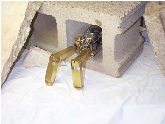
Figure 1. Image of CRAWLER Scout emerging from a cinder block using a modified narrow-passage gait.
