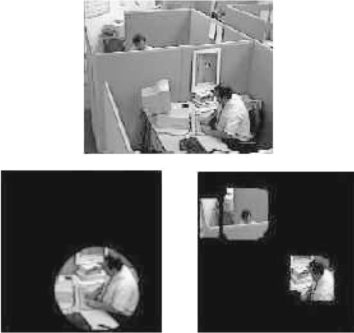
Fig. 11.1. Human vs. machine novelty. The top image is the original video frame depicting an office scene where an employee is typing things into a computer. The image on the lower left depicts the novelty component found by a human subject in the study using an eye tracker. The image on the lower right is the novelty as determined automatically by a machine vision system we developed (termed VENUS). The two novelty components for the same video frame show that both the human and machine can find similar parts to be novel.
