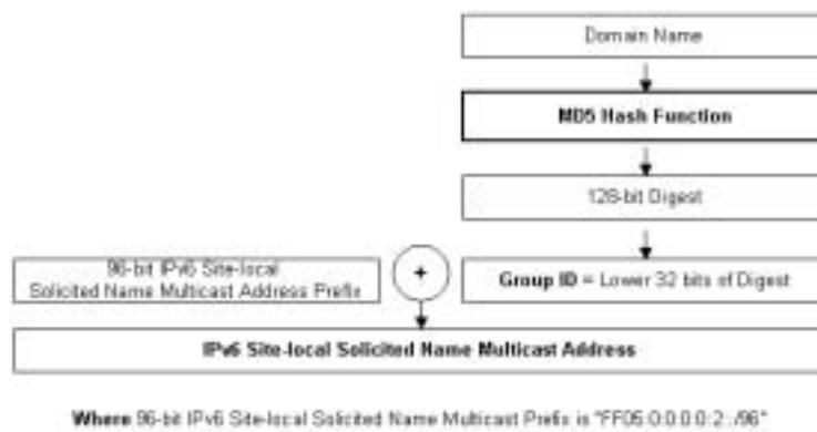
Fig. 7. Generation of IPv6 Site-local Solicited Name Multicast Address
