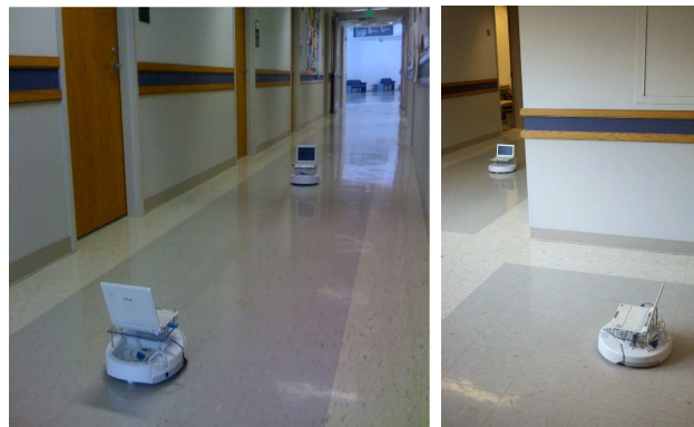
Fig. 8. LEFT: Experiment setup for the first and second groups showing two iRobot Create robots equipped with Asus EEE PC laptop on it placed on a straight corridor. RIGHT: Experiment setup for the third group showing two iRobot Create robots equipped with Asus EEE PC laptop on it placed on a rectangular shaped corridor in an indoor environment.
