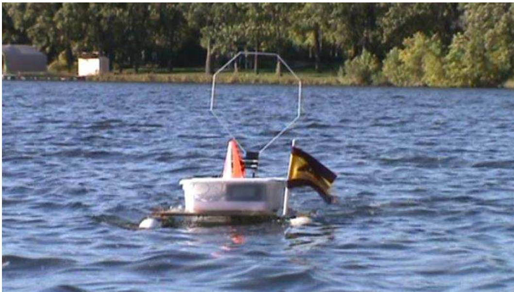
Figure 1: The raft during field trials at Lake Phalen. A directional loop antenna which records signals from radio tagged fish is attached to a pan-tilt unit on top of the raft.
