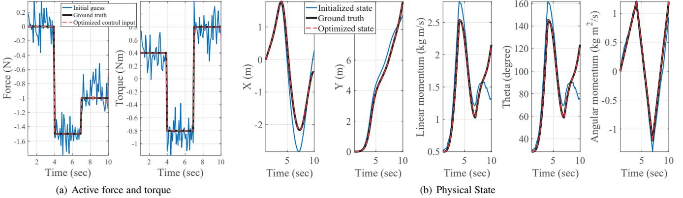
Fig. 8. We compute the optimal control (a) and its state (b) using Equation (12) that minimizes reprojection error for a synthetically generated motion. Given a camera trajectory, we initialize control input and then, compute the initial state (blue) using Equation (14).
