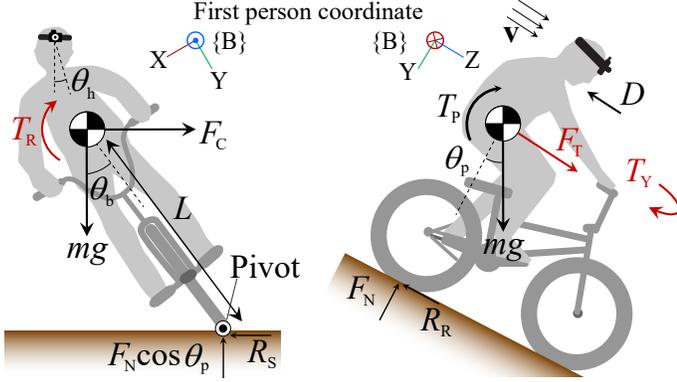
Fig. 3. We model the actor's dynamics using an inverted pendulum where the force and torque are decomposed into two components: passive components (weight,  $mg$ ; centripetal force,  $F_C$ ; normal force,  $F_N$ ; sliding and rolling friction force,  $R_S$  and  $R_R$ ; air drag,  $D$ ; pitch torque,  $T_P$ ) and active components (thrust,  $F_T$ ; roll torque,  $T_R$ ; yaw torque,  $T_Y$ ).
