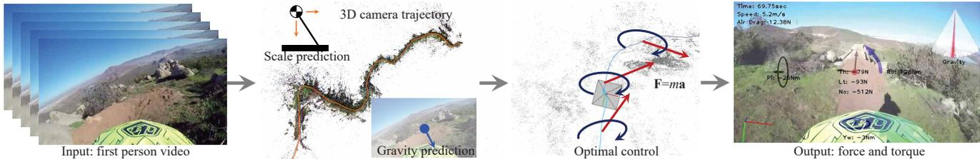
Fig. 2. Our system takes a first-person video of sporting activities and estimate the active force and torque that generates the camera ego-motion. We recognize a physical metric space by estimating gravity and metric scale. Based on the coordinate, we compute the optimal force acting on the actor’s body by minimizing reprojection error.
