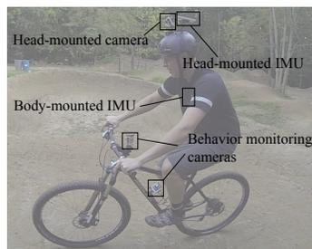
Fig. 12. Controlled experiments with an experienced mountain biker.
