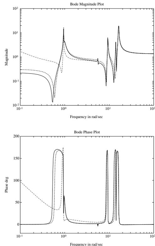
**Figure 3** Bode Plots of (1,1) Transfer Function: Full order model (solid); Matrix Pencil (dashed); Balanced Realization (dash-dot).
