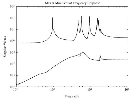
**Figure 1** Max & Min SV's: Matrix Pencil Approach (dashed); Full order model (solid).
