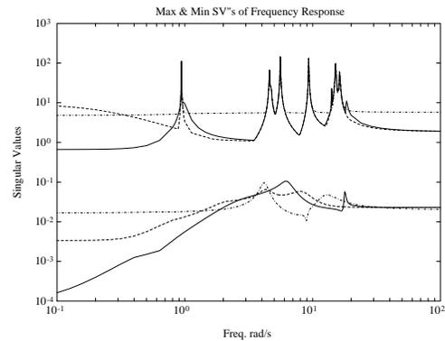
**Figure 2** Max & Min SV's: Full order model (solid); Balanced Realization (dashed); Hankel Norm (dash-dot).
