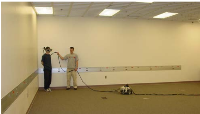
Figure 3: A photograph of a participant at the starting point of the 30' distance interval wearing the head mounted display and tracking sensor, with an assistant managing the cables. The second sensor, which is not used during the walking trials, can be seen resting on top of the cart-mounted video control unit. Tape marks indicating the starting points of the 10' and 20' intervals can be seen on the floor to the right of the video control unit.
