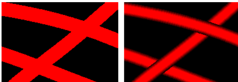
Figure 4. Left: Overlaid streamlines result in an image in which it is difficult to determine distinct streamlines. Right: A textured halo around the streamlines gives each streamline a 3D appearance and also creates discontinuity between overlapping streamlines.
