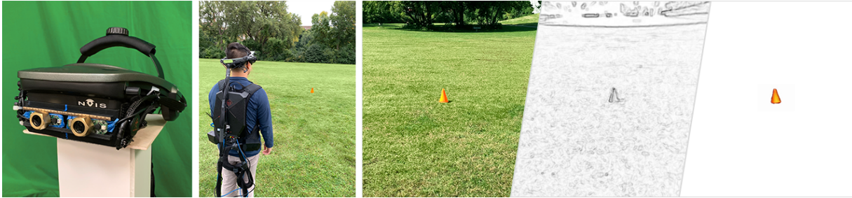
Figure 1: Left to Right: (1) Custom 3D-printed visor with adjustable cameras and neutral-density lens filters, mounted on an optical-see-through head-mounted display. (2) Equipment in use, with portable backpack computer. (3) Gradual reduction of scene detail: raw camera view, Sobel filtered camera view (non-photorealistic style), and full background subtraction (target only).
