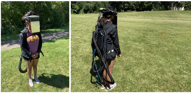
Figure 6: Left: HMD with flapper to block the participant's view in the real-world viewing condition ( M_{RW} ). Right: M_{RW} trial at L_3 location.
