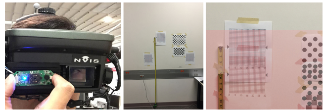
Figure 3: Left: Enabling the bi-ocular viewing; Middle: the optical view; Right: a zoomed-in illustration of the superposition of the camera view (tinted pink).
