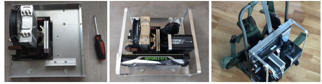
Figure 4: Mounting parts on the custom back-plate, and final backpack computer (without cover) on the ALICE frame.
