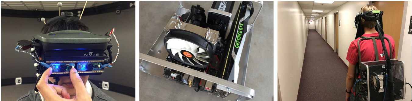
Figure 1: Left: 3D-Printed visor with adjustable cameras. Middle: Custom backpack computer. Right: Final system in use.
