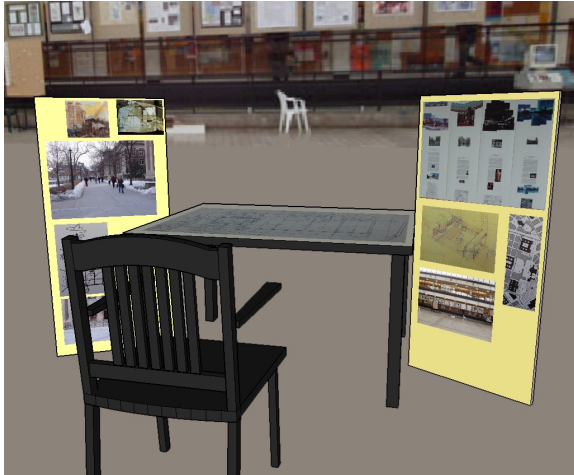
Figure 8: A closeup view of the DesignStation in the virtual design environment, in which images, videos, sketches and other material relevant to the design task are visually accessible on two flanking displayboards.
