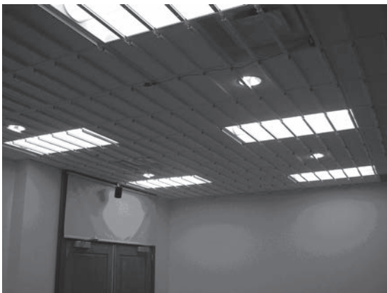
Figure 2. A picture of the diode strips for the optical HiBall tracking system mounted on the ceiling in our lab.
