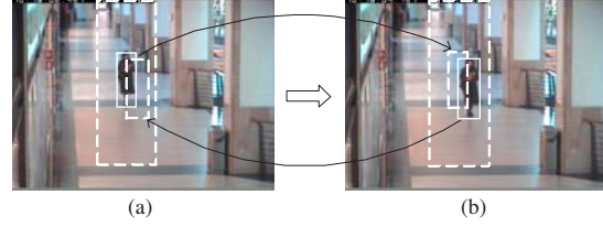
Figure 3. DEMD tracking with background modeling (a) The (t-1)^{th} frame (b) The t^{th} frame. Pixels within the solid-line rectangle belong to the object, pixels outside the solid-line rectangle and within the larger dashed-line rectangle belong to the local background. For the ideal object scale and position in the t^{th} frame, the object should conform to its model; besides, the local background region, i.e., the area outside the two foreground regions and within the background region of the t^{th} frame, should match the same area of the previous frame.
