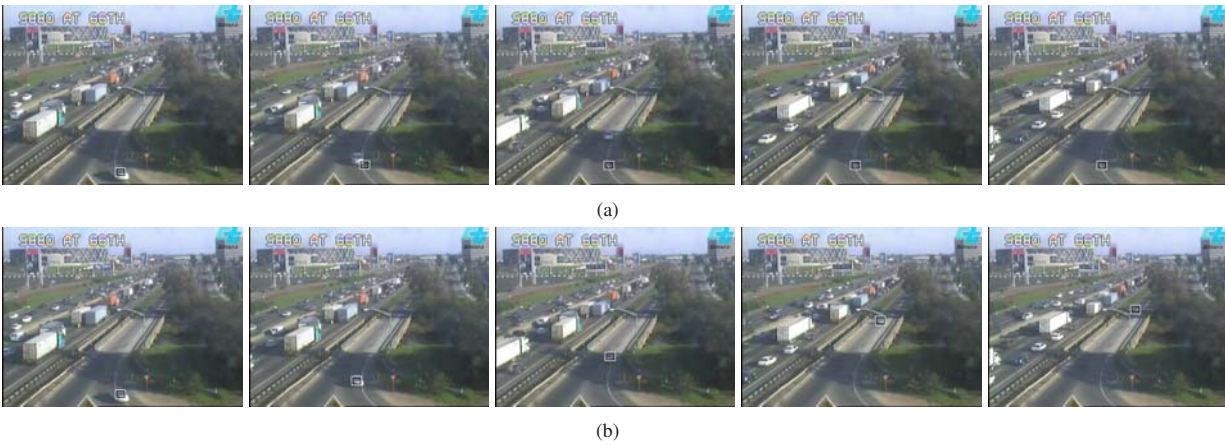
Figure 5. Frames 1, 13, 35, 86, 110 from the Highway-Car sequence. (a) The MS tracker starts to wander when the car is entering the strong shadow and fails around frame 13. (b) The DEMD tracker successfully follows the car into and out of strong shadows.
