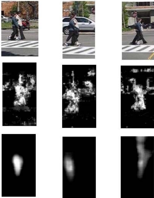
Figure 3. A comparison of our confidence maps with those of the Ensemble Tracker. Original frames are given in the top row. The middle row contains the confidence maps generated by the Ensemble Tracking algorithm. The bottom row shows the confidence maps generated by our algorithm.
