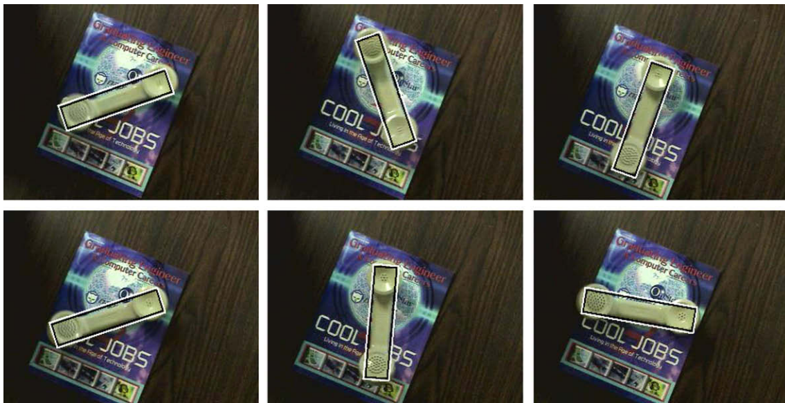
Fig. 13. Handset sequence: the SCC based tracker successfully tracks the object despite of wide rotation of the object.
