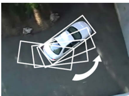
Fig. 1. SCC based tracker. Orientation of an object is estimated simultaneously with its position.
