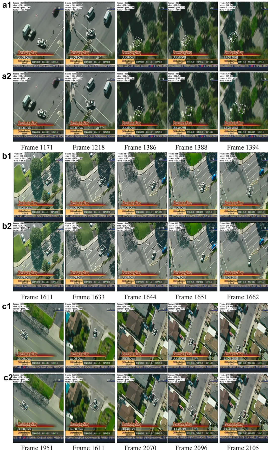
Fig. 7. Car-chasing sequence: (a-1, b-1, c-1) the optimal SCC based tracker tracks the car throughout the 2250 frames. (a-2) Non-optimal SCC based tracker fails during partial occlusion. (b-2, c-2) The MS tracker loses track of the object when (b-2) the car makes turns, (c-2) background scene is cluttered.
