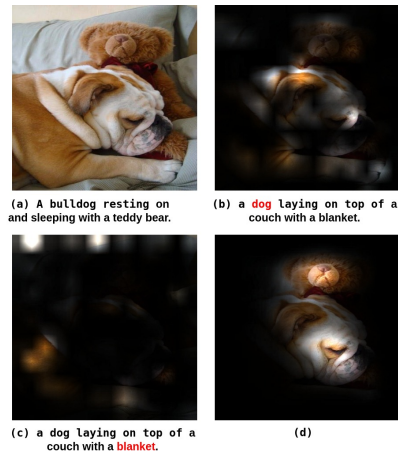
Fig. 1. Top-down attention may fail to focus on objects of interest. (a): original image with human-generated caption, (b-c) two top-down attention maps and their corresponding model-generated captions, and (d) stimulus-based attention map for the image. Words related to the top-down attention maps are colored in red.
