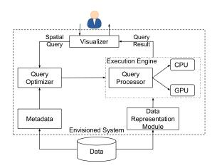
Fig. 2: System Architecture
