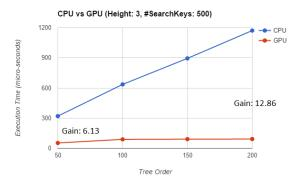
Fig. 3: Effect of index size on execution time
