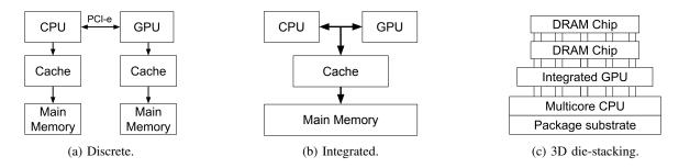
Fig. 1: CPU-GPU architectures
