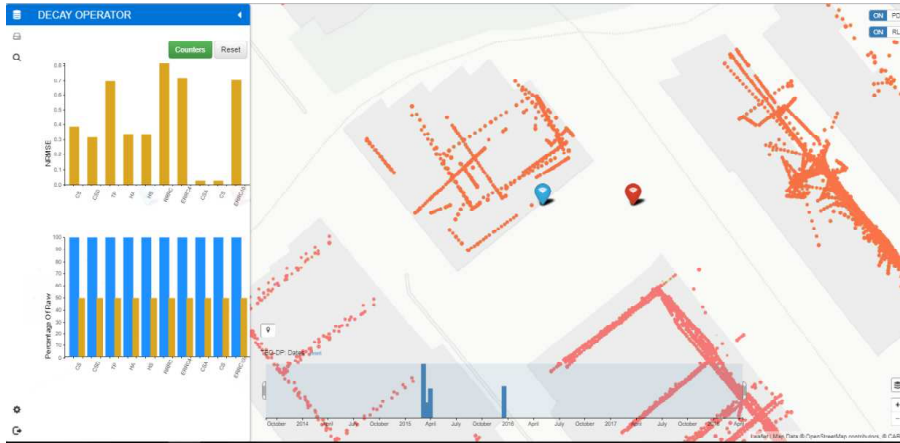
Fig. 7 The TBD-DP operator implemented inside the spatio-temporal SPATE architecture. The interface enables users to carry out high resolution visual analytics, without consuming enormous amounts of storage. The savings are quantified numerically with bar charts and visually with heatmaps.
