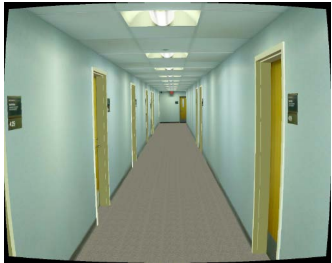
Figure 2: The model of the virtual hallway as seen through the head mounted display. Pincushion distortion caused by the lenses in the head mount is corrected by a barrel-distortion post process.
