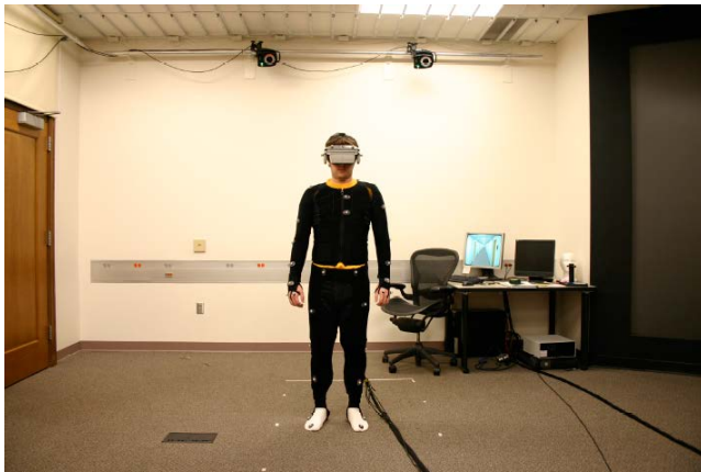
Figure 1: The Vicon tracking apparatus. This shows the user wearing the black suit with 1cm spherical markers placed on their limbs. A pair of Vicon cameras can be seen mounted on the bars near the ceiling of the lab.
