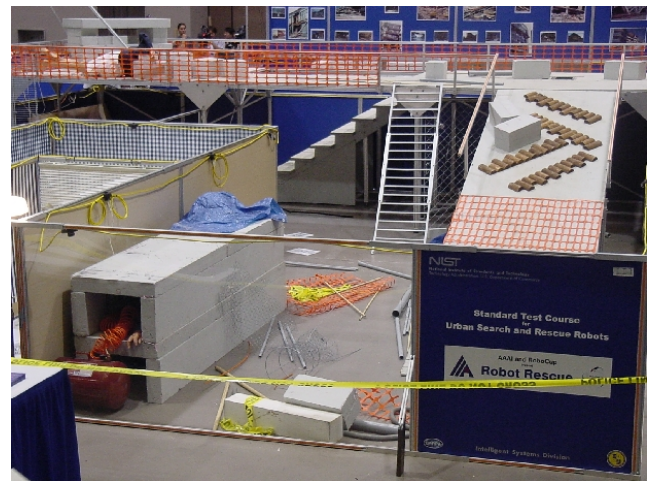
Figure 1: Part of the IJCAI Urban Search and Rescue Course. This course was constructed by NIST and was designed to simulate an urban disaster area. Teams earned points for locating and correctly identifying “victims” as well as notifying human operators of the victims’ locations.
