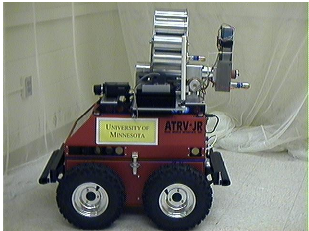
Figure 2: A ranger robot with scout launcher.
