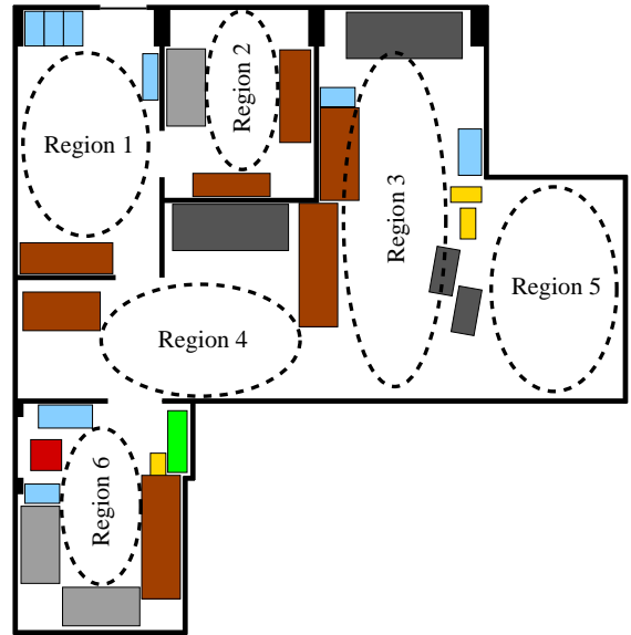
Fig. 19. A top-down view of a complex (multi-room) environment and how it could be broken into multiple smaller convex regions. Each region would have its own Scout (or set of Scouts) to monitor it.
