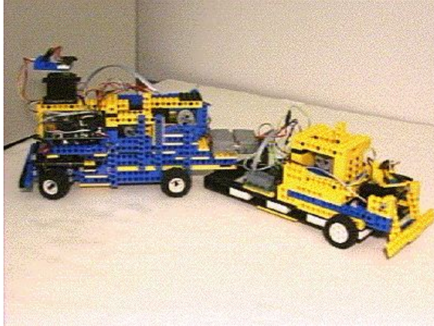
Figure 7: The Self-Positioning Trailer-Backing Mini-robot.
